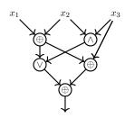
Figure 2: A circuit that takes 3 bits as input and has depth 3. If f is the function computed by this circuit, then you can check that, e.g., f(1,0,1) = 0 and f(1,1,1) = 0. (Thanks to Sasha Golovnev for the figure.)
