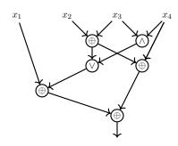
Figure 1: A circuit with four-bit input and depth 3. If f is the function computed by this circuit, then you can check that, e.g., f(1,0,1,0) = 1 and f(1,1,1,1) = 0. (Thanks to Sasha Golovnev for the figure.)
